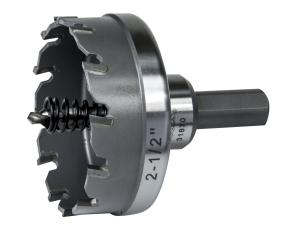
This carbide hole cutter cuts quick, precise holes in a variety of materials. Integrated flange prevents the operator from drilling beyond the sheet metal. Split point pilot drill bit prevents bit walking.
