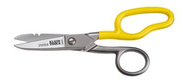
These Free-Fall Snips feature high carbon steel blades to cut 19 AWG and 23 AWG electrical communication wire. They also strip 19 AWG and 23 AWG wire. The extended handle provides comfort and cutting leverage for wire cutting applications. The blades are made of high carbon steel blade (58 HRC) to maintain blade durability and sharpness. Serrated teeth allow for non-slip cutting action. The free-fall feature provides a looser fit.
