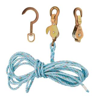
All Klein block and tackle use high-quality, 3/8-Inch (10 mm) diameter rope. Light, galvanized-steel shell blocks are fitted with snubbing hooks to hold the load. This package features two blocks with a swivel Klein hook Cat. No. 259 with a maximum safe load of 750-pound (340 kg).
