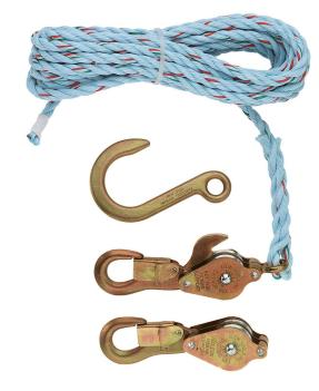
Light, galvanized-steel shell blocks are fitted with snubbing hooks to hold the load. Sheaves are strong yet lightweight aluminum alloy with all-bronze bushings. Available with standard snap hooks or guarded snap hooks (with snap hook nose lengthened to extend over the latch or keeper).
