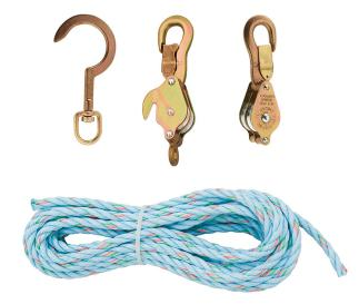
All Klein block and tackle use high-quality, 3/8-Inch (10 mm) diameter rope. Light, galvanized-steel shell blocks are fitted with snubbing hooks to hold the load. This package features two blocks with a standard swivel anchor hook with a maximum safe load is 750-pound (340 kg).
