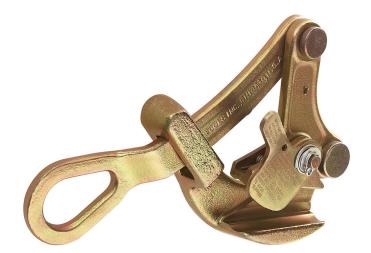
Lightweight, compact grips pull an exceptionally wide range of cable sizes and types. Designed with a round inside-jaw contour for maximum contact to minimize conductor damage. Lower jaw is serrated to firmly grip insulated cables and conductors. Design includes a latch that prevents the grip from falling in case of jaw disengagement from the cable.
