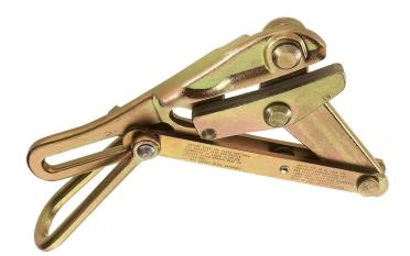
Designed for use on aluminum, copper, weatherproof coated wire, PVC covered conductors and messenger and guy strand. The Chicago style grip was designed for cable sizes from 0.12-Inch to 1.0-Inch (3.10 to 25.4 mm). When pulling EHS (extra-high-strength) galvanized-steel cable, the galvanizing has a tendency to coat the jaws of any grip, causing the cable to slip. Double V contour reduces the possibility of slippage and damage to the cable.
