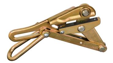
Designed for use on aluminum, copper, weatherproof coated wire, PVC covered conductors and messenger and guy strand. The Chicago style grip was designed for cable sizes from 0.16-Inch to 0.55-Inch (4.06 - 13.97 mm). Double V grooves give four-point contact, reducing chance of slipping and providing proper alignment of wire and cable.
