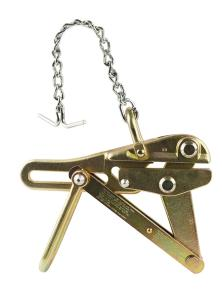
This Chicago Grip is designed specifically to work with coated guy strand and EHS cable. Klein grips are made of drop-forged, quality US steel and heat treated for strength and durability. The chain, toggle and shackle keep the grip from falling off the cable. The 5-Inch jaw length increases the surface area contact with the cable minimizing cable damage. The sawtooth jaw profile resists galvanization build-up.
