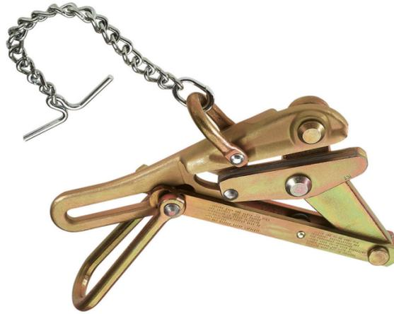
Designed for use on aluminum, copper, weatherproof coated wire, PVC covered conductors and messenger and guy strand. Identical to Bell-System type L strand puller. Equipped with chain, toggle and shackle. For support wire 0.134-Inch and larger, refer to 1659 series. Outside diameter of support wire includes thickness of polyethylene coating.
