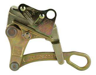
This lightweight, compact grip pulls ACSR cable from 0.16 to 0.90-Inch (0.4 to 2.3 cm) in diameter. The round jaw provides maximum contact with the cable while minimizing deformation. The hot latch closes automatically to guard against the grip accidentally disengaging from wire. This model features a locking handle to keep the jaw open while the grip is placed on the cable with a hot stick.
