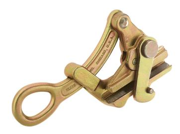
The Klein Tools 1671-10 Parallel Jaw Grip works with a wide range of cable types and sizes. The longer jaws provide a firm hold on the cable, reducing the possibility of slippage and deformation. All Klein grips are manufactured from custom drop-forged steel that is machined and heat treated for excellent durability. Each grip is individually hand inspected and actuated for proper function. Grips are also rigorously tested and pulled to rated load to ensure the highest quality and reliability.
