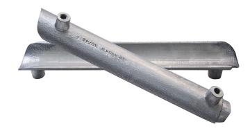
This Klein Tools Interchangeable Grip Liner is designed to be used with Klein Tools' 1628-60 Interchangeable Grip. These grip liners are removable and can be switched out with 12 other jaw liners to make the 1628-60 grip compatible with multiple sizes of ACSR, ACSS, and AAC cables. These interchangeable liners are inserted between the upper and lower jaws of the grip to keep cable securely in place.
