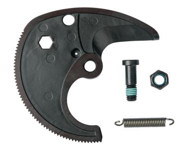
Replacement blade set for Klein's 63607 (2017 Edition) Ratcheting ACSR Cable Cutter. Hardened steel blades cut up to 600 MCM Copper and 750 MCM Aluminum. Set includes moveable cutting blade, fulcrum screw, lock nut for fulcrum screw.
