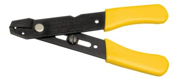
Klein Tools' 1003 Wire Stripper and Cutter is a handy, light, compact tool for stripping 12-26 AWG solid and 14-28 AWG stranded wire. Features convenient hole for looping or bending wire. Adjustable slide stop with set screw for repeat stripping work.
