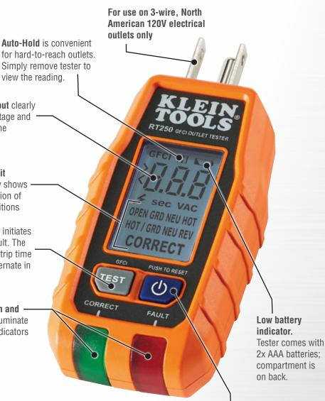
CLEAR INDICATION OF VOLTAGE AND WIRING CONDITIONS
