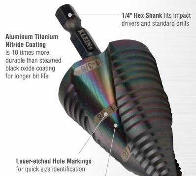
**Dual Spiral Flutes** pull bit through material for faster cuts
