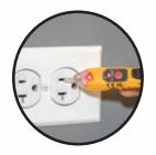
When voltage is detected, a high intensity, bright red LED illuminates and an audible tone will sound
