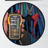
MAP WIRES TO Check Pin-to-Pin Connections
