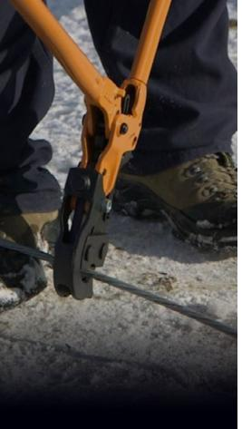
The Heavy-Duty Ratcheting **Bolt Cutter easily slices** through guy strand in just one cut. A smooth ratchet mechanism makes this bolt cutter the easiest to use on the market.
