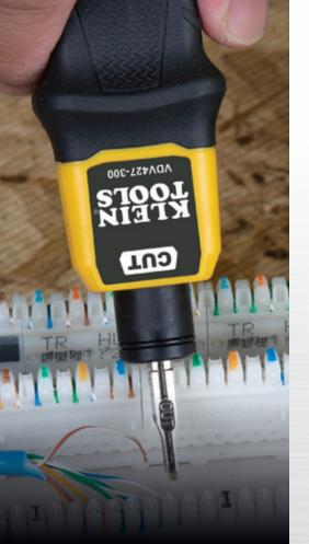
TERMINATE AND CUT WIRES IN ONE STEP PUNCH CABLES INTO 66/110 PANELS AND BLOCKS
