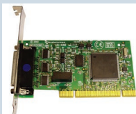
UC-083 uPCI 4xRS232 Opto Isolated TX RX GND CTS RTS
