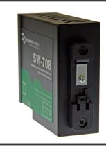
Integral DIN mount and slim design provides Ethernet connection to multiple devices
