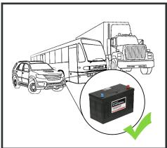
+5 to +30 Volt Power Input enables the device to be run from a standard car battery ideal for in vehicle applications
