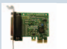
PX-157: LP PCIe 1xLPT Printer Port
