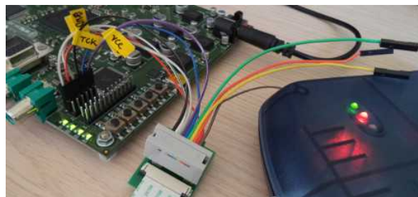
Figure 18: ATmega programming set-up using the JTAG header
