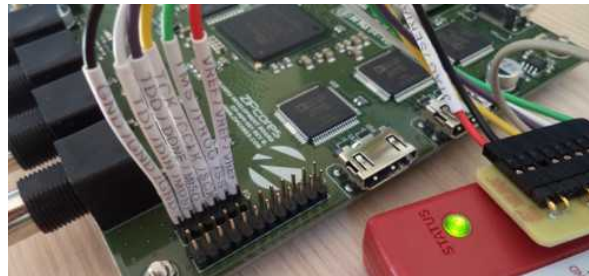
Figure 17: FPGA programming set-up using the JTAG header
