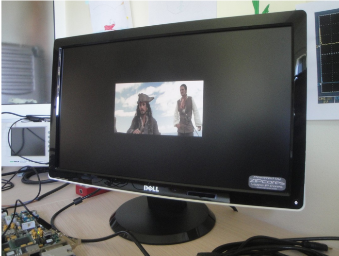
Figure 7: Scaler demo lab setup (Generation of a small 500x400 video window on SXGA background)
