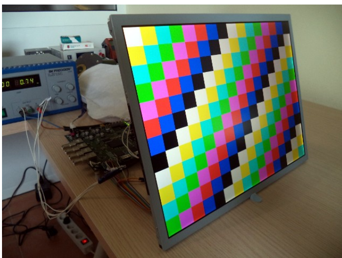
Figure 7: LVDS demo showing Sharp LCD (WXGA) test pattern display
