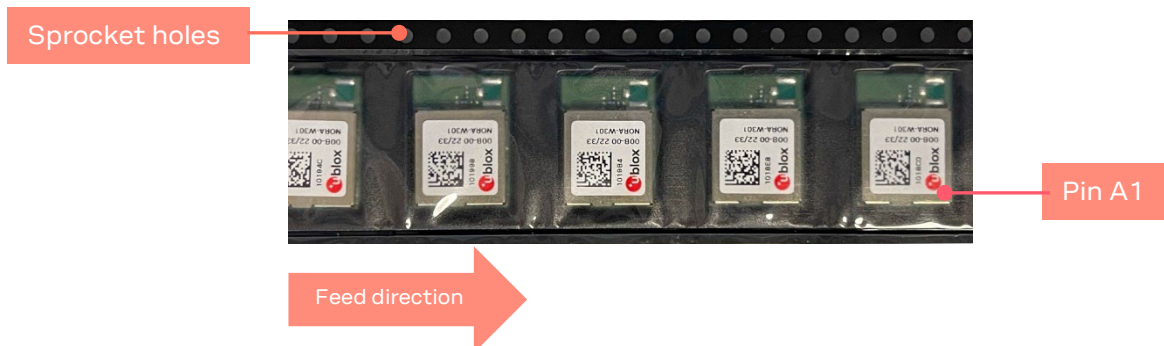
Figure 7: NORA-W361 module on tape orientation
