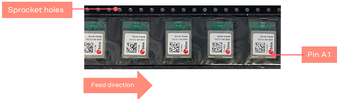
Figure 8: NORA-W366 module on tape orientation
