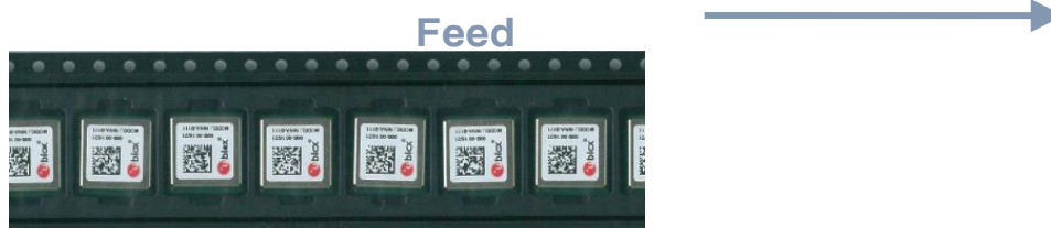
Figure 12: Orientation of NINA-W151 module on tape
