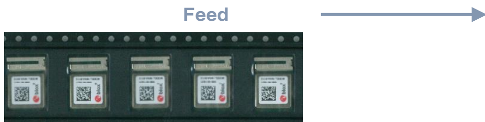
Figure 13: Orientation of NINA-W152/NINA-W156 module on tape
