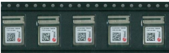
Figure 12: Orientation of NINA-W132 module on tape
