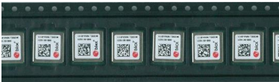
Figure 11: Orientation of NINA-W131 module on tape
