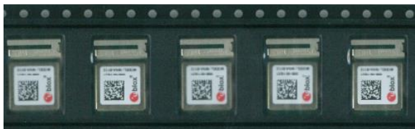
Figure 12: NINA-W102/NINA-W106 module on tape orientation
