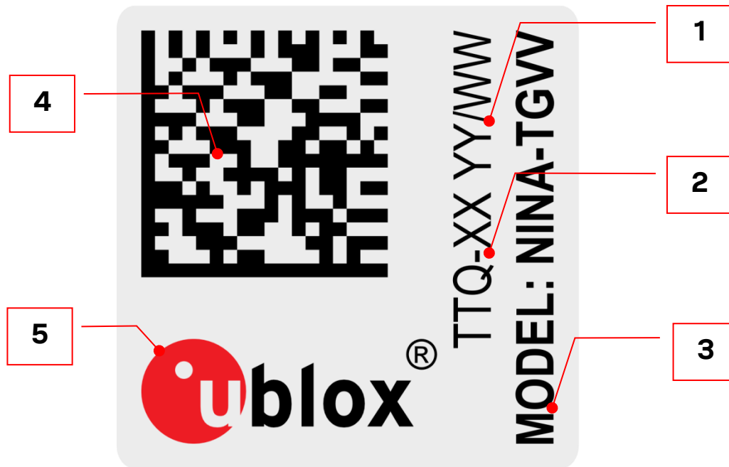
Figure 15: Location of product type number on the NINA-W10 series module label
