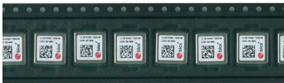
Figure 11: NINA-W101 module on tape orientation
