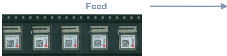
Figure 11: Orientation of NINA-B222 module on tape
