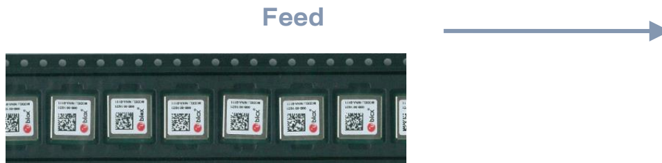
Figure 10: Orientation of NINA-B221 module on tape
