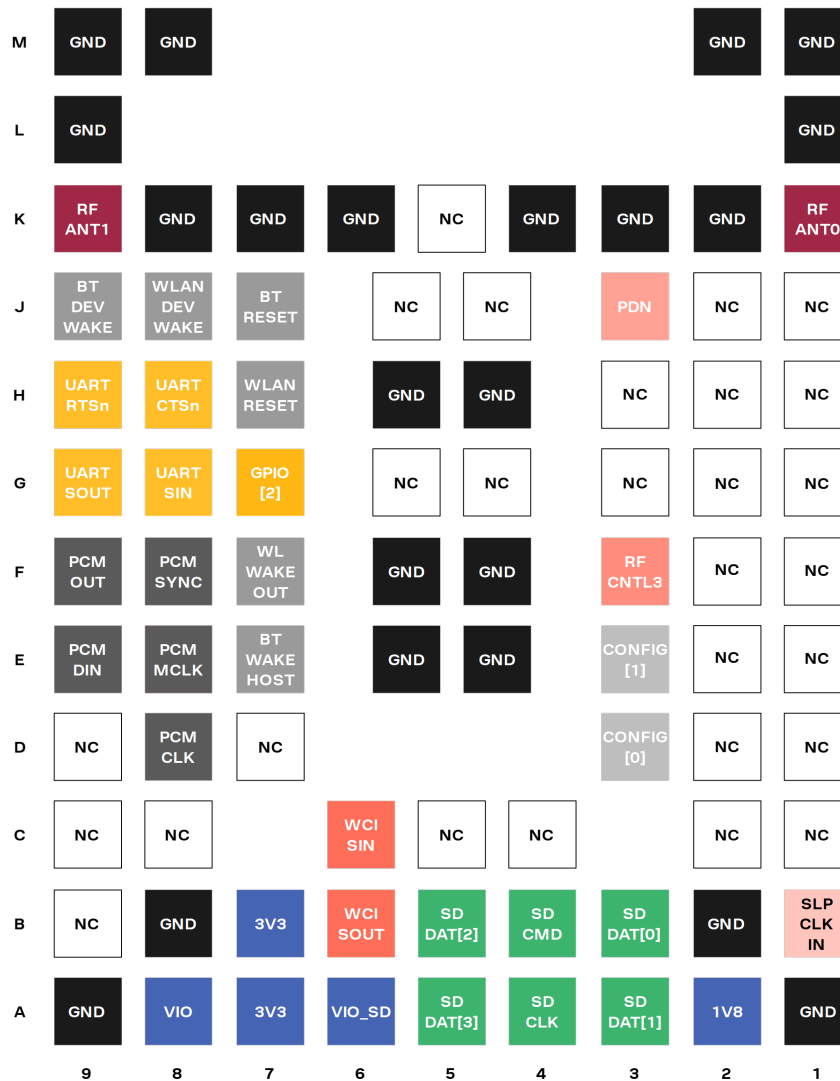
Figure 13: MAYA-W1 series pin assignment (top view)
