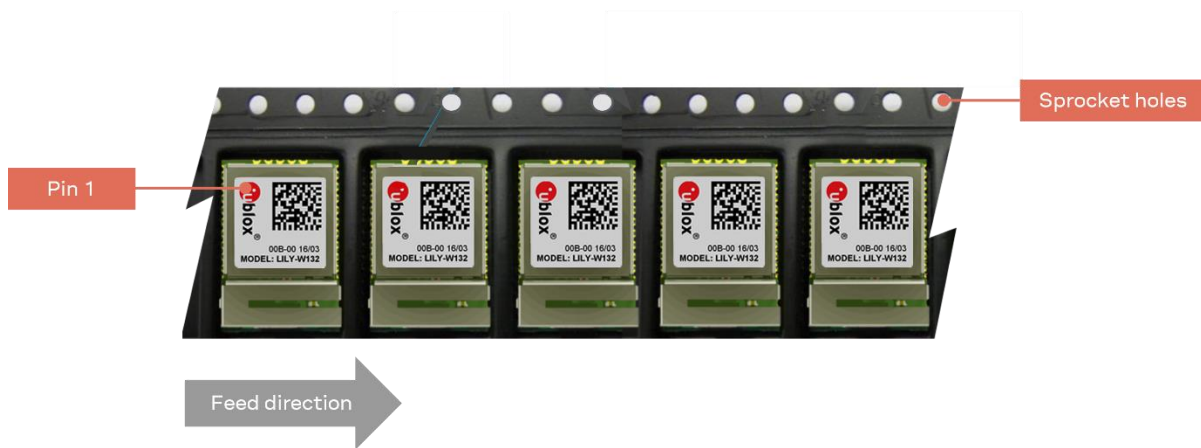
Figure 7: Orientation of LILY-W132 modules on tape
