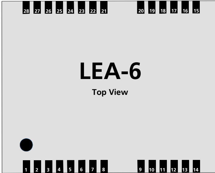
Figure 2 LEA-6 Pin Assignment
