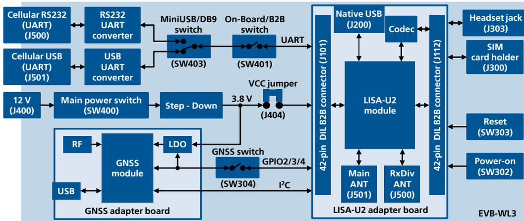
Figure 2: EVK-U2x block diagram
