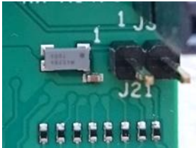
Figure 9: 32.768 kHz oscillator and pin header J21
