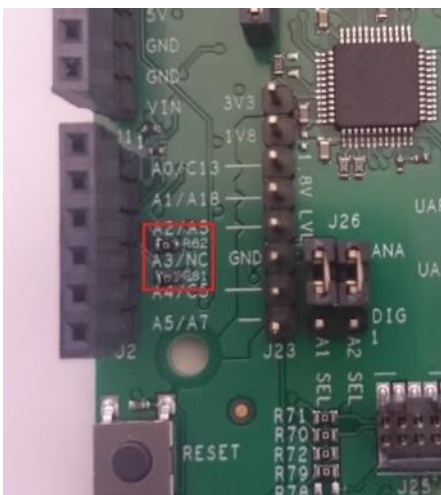
Figure 8: Resistors R81 and R82
