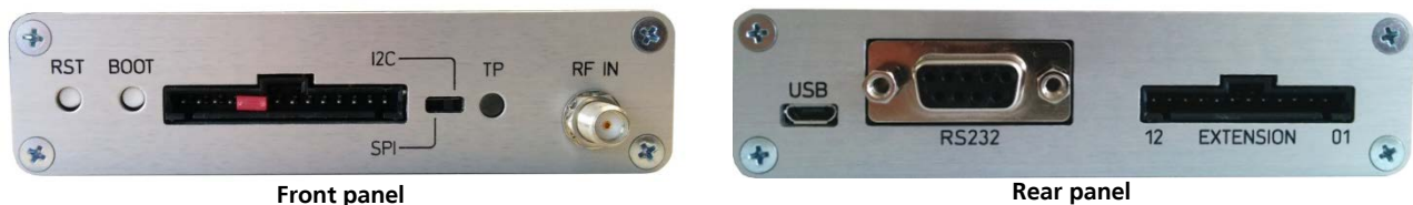
Figure 2: EVK-M8F-0-00 evaluation unit – front and rear panels
