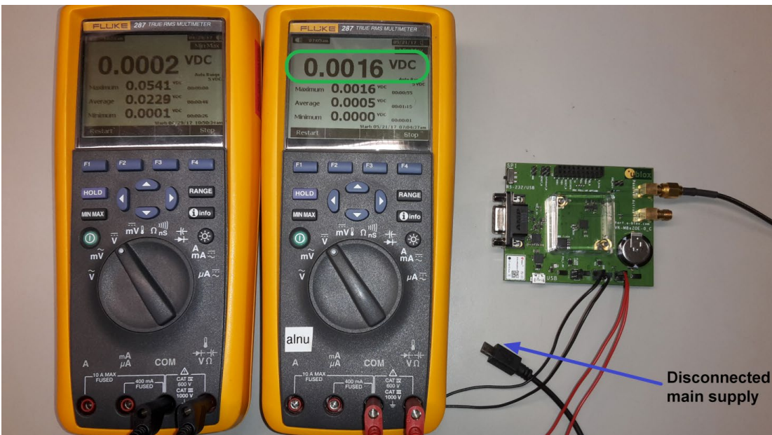
Figure 11: Setup to measure the V_BCKP current consumption of ZOE-M8B on EVK-M8BZOE
