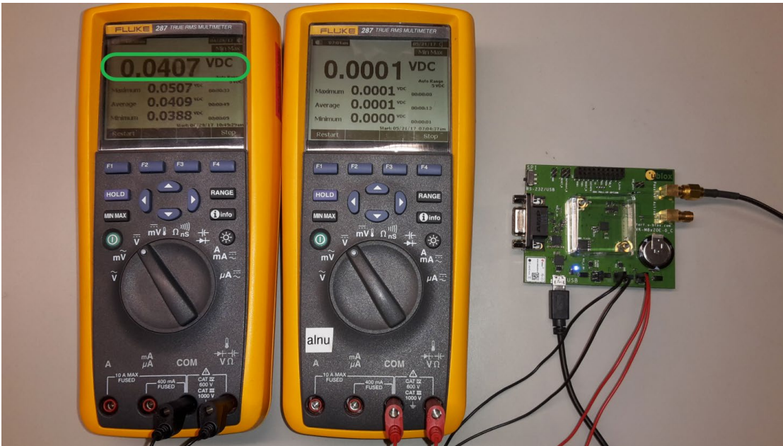
Figure 10: Setup to measure the VCC current consumption of ZOE-M8B on EVK-M8BZOE
