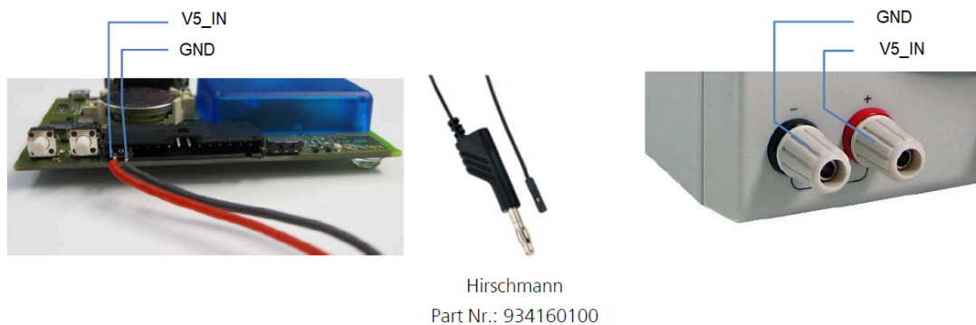
Figure 3: EVK-M10QSAM 5.0 V DC power supply example
