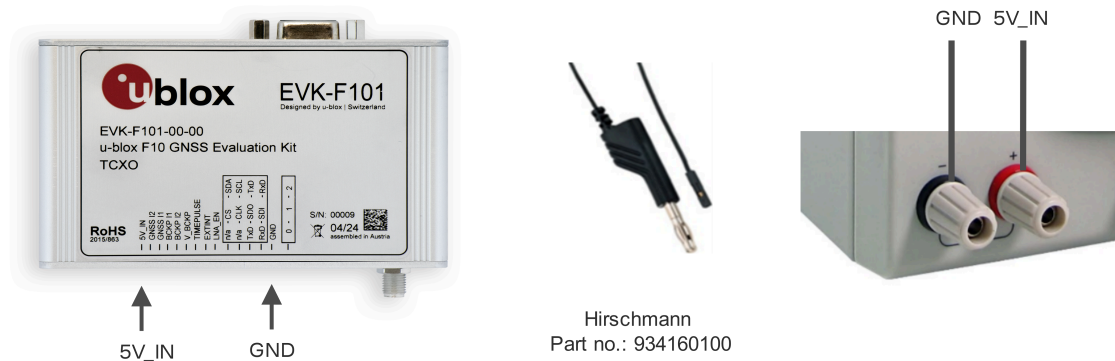
Figure 3: EVK-F101 5.0 V DC power supply example
