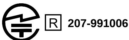
Figure 14: Giteki mark, R and the EMMY-W163 MIC certification number. The "Indoor use only" information translated into Japanese below is mandatory if the product is operating in the 5.2/5.3 GHz band.
