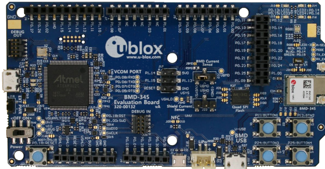
Figure 1: EVK BMD-345 evaluation board (Top view)
