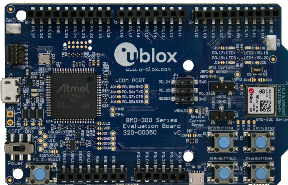
Figure 1: BMD-3xx-EVAL User Guide evaluation board (top view)
