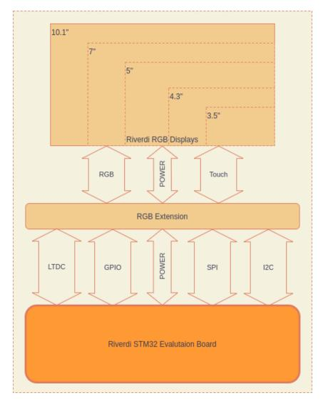
Caution: So far, 10.1" displays are available with LVDS interface, 7.0" displays with either LVDS or RGB interfaces, and all the rest (3.5", 4.3" and 5.0") with RGB interface as standard.
