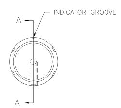
USE #28 DRILL (0.140), #8-32 TAP, #8-32 X 1/4 LG. CUP POINTED, SLOTTED TYPE, SET SCREW 10357 (1)
