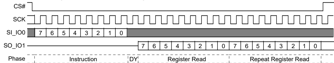
Figure 111. Protection Register Read (PRRD) Command Sequence
