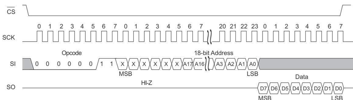
**Figure 13. Fast Read Operation**
