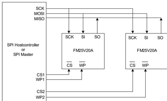
**Figure 4. System Configuration without SPI Port**
